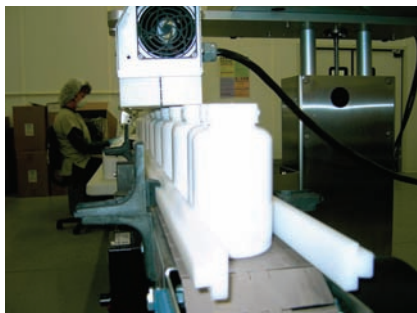
New Life shuttles the induction sealer between its two bottling lines. The company plans to purchase a second induction sealer once production volume justifies it.
