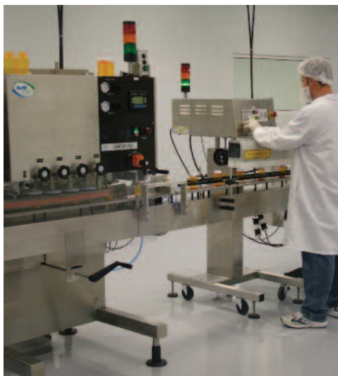
You need 3 to 5 feet of straight, unimpeded conveyor for mounting or placing the sealing coil.
